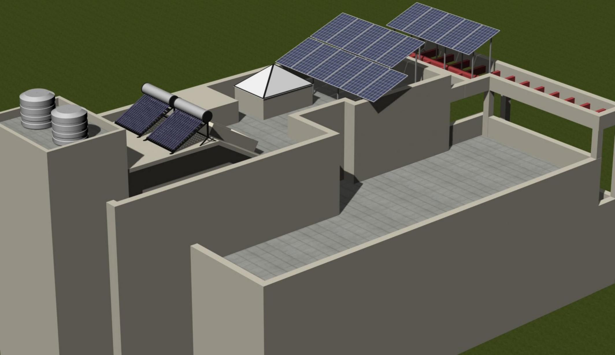
Proposed 5 kwp Solar PV system at Nanded
